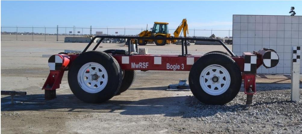
Figure 1. Rigid-Frame Bogie on Guidance Track
